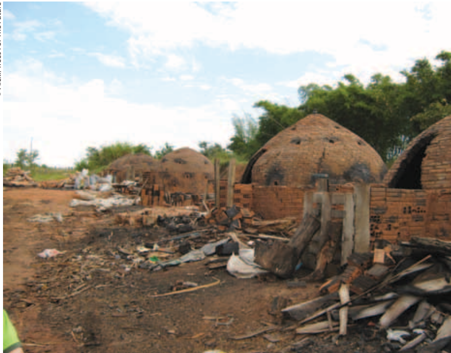
Charcoal is created by burning logs in a low-oxygen environment using mounds of earth or kilns, such as these in Brazil
